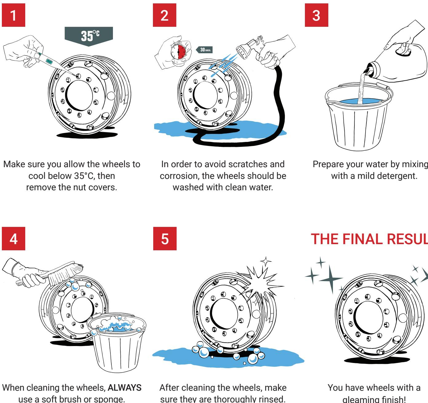
Make sure you allow the wheels to cool below 35°C, then remove the nut covers.
