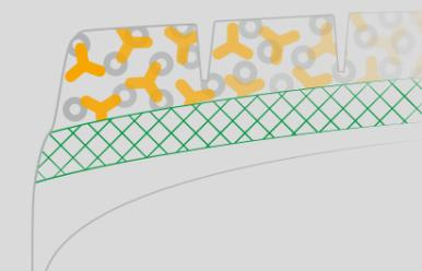
Adjusted outer groove positioning\* for improved tread integrity
