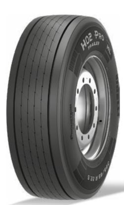
The latest generation of trailer tyres for long-haul transport designed for maximum efficiency and for fleet operating costs optimization. Low rolling resistance, great wet braking performance and high load capacity.
