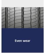
New pattern geometry featuring innovative high density and full depth wave sipes
